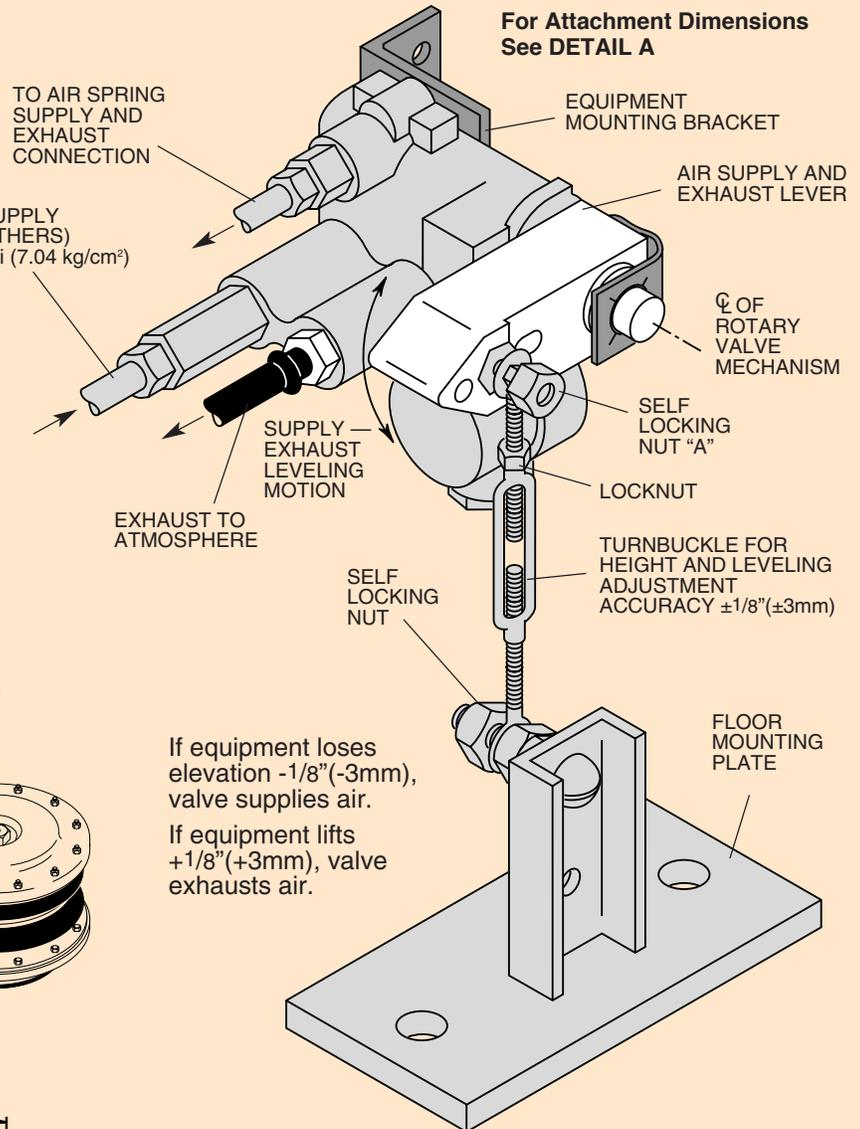
If equipment loses elevation  $-1/8"$  ( $-3\text{mm}$ ),
