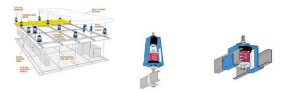
Floating Floors remain the most effective way of reducing sound transmission and vibration from the floor above. However, there are many situations where a floating floor is impractical or not economically feasible, so an isolated ceiling becomes the practical choice.
