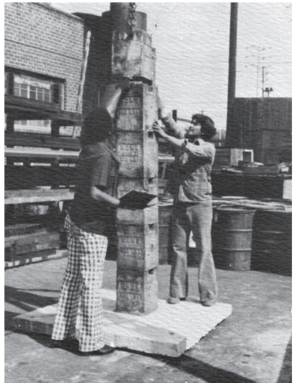
Applying 3000 lb concentrated load to Test Slab 1.
