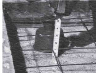
Mount in photograph was placed on 48" centers with 6 x 6 mesh cut for test purposes only. Sketch shows the normal stronger position in center of 6 x 6 square.
