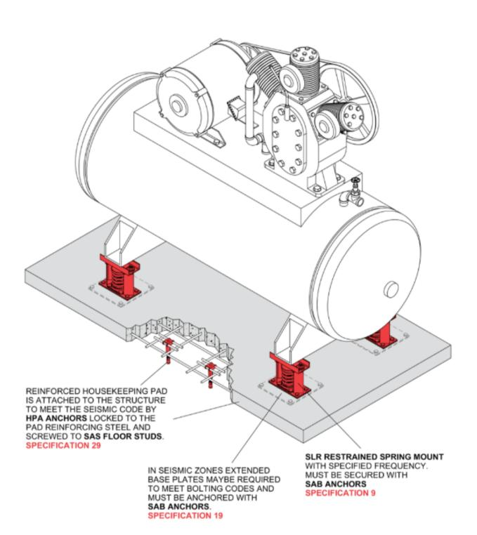
RECIPROCATING DIRECT DRIVE COMPRESSOR with height saving brackets on high deflection SLF Mounts and Z-1011 Seismic Restraints. Reinforced housekeeping pad secured by HPA Anchors.
