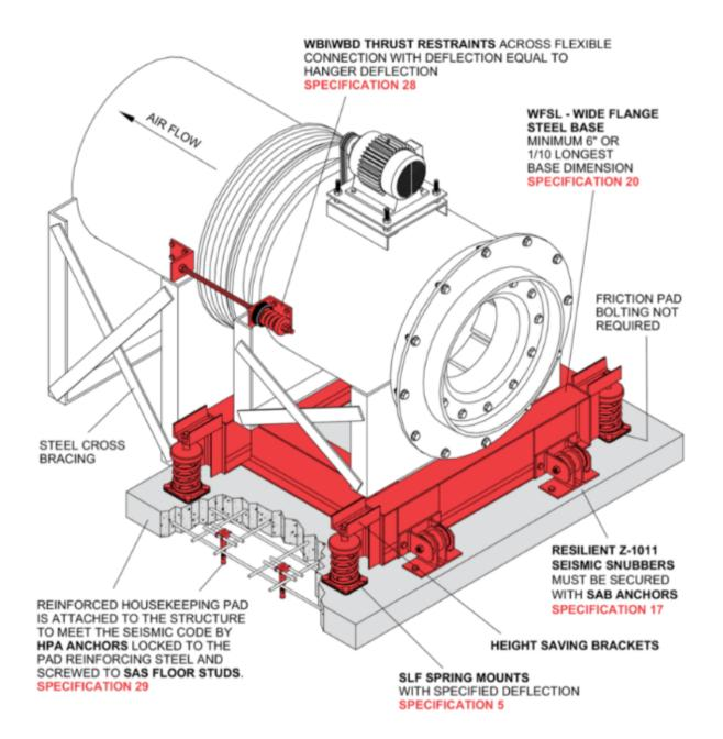
CENTRIFUGAL BLOWER on concrete filled BMK Base with built in corners, 1" deflection SLF Spring Mounts and Z-1011 Seismic Restraints. Reinforced housekeeping pad secured by HPA Anchors.
