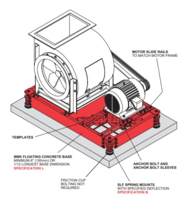
**CENTRIFUGAL BLOWER** on concrete filled BMK Base with height saving brackets and high deflection SLF Spring Mounts
