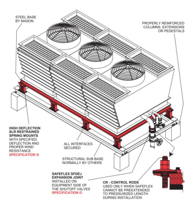
PACKAGED HVAC COOLING TOWER on steel base with SLR-MT wind resistant Twin Sphere Air Spring Mounts. SAFEFLEX Expansion Joints are installed in pipelines to reduce blade frequency vibration and noise
