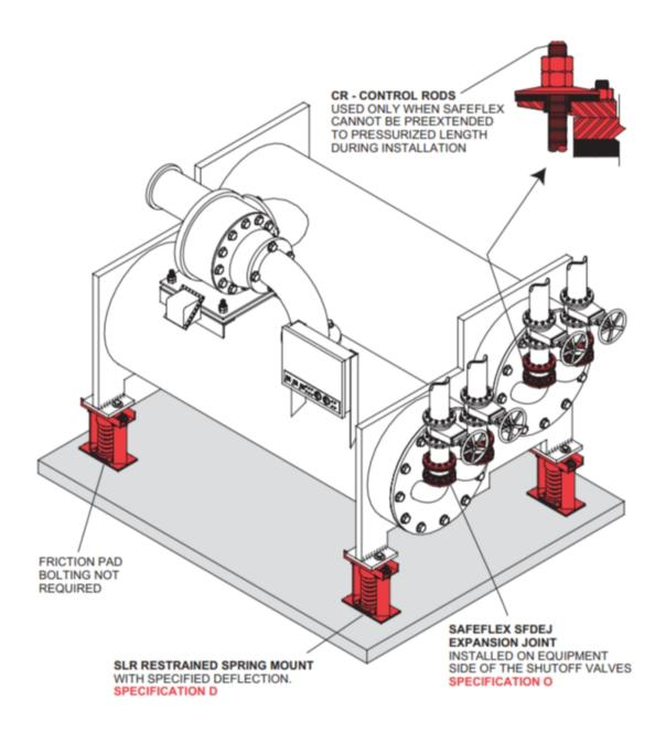
CENTRIFUGAL CHILLER directly mounted on SLR-MT Restrained Twin Sphere Air Spring Mounts to simplify rigging and maintain emergency elevation. SAFEFLEX Expansion Joints are installed in pipelines to reduce blade frequency vibration and noise.
