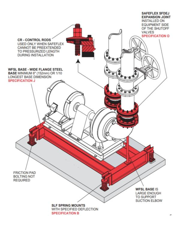
**END SUCTION PUMP** on WFSL Base and MT Air springs spring mounts. SAFEFLEX Expansion Joints are installed in pipelines troeduce blade frequency vibration and noise.
