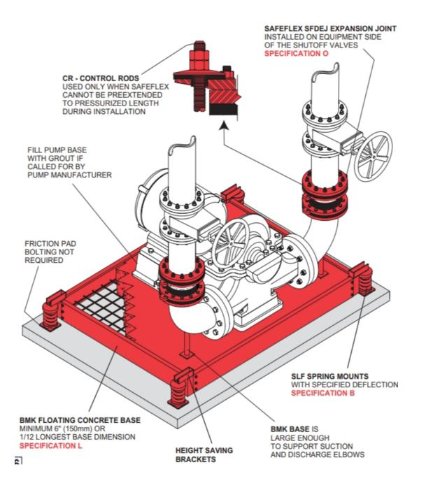
**END SUCTION PUMP** on WFSL Base with height saving brackets and high deflection SLF spring mounts. SAFEFLEX Expansion Joints are installed in pipelines troeduce blade frequency vibration and noise.
