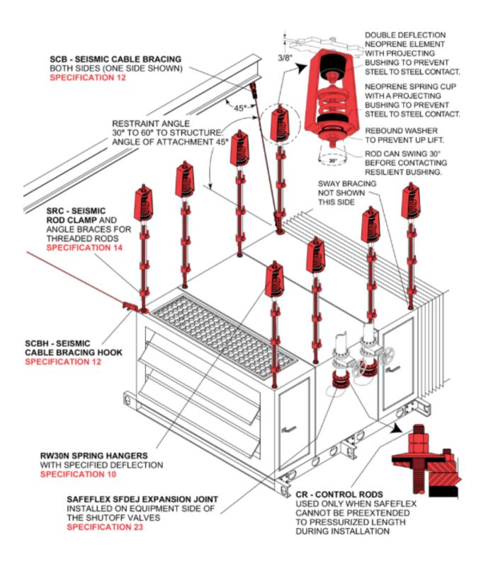
HVAC UNIT on steel base with height saving brackets, high deflection SLF Spring Mounts and Z-1011 Seismic Restraints. Reinforced housekeeping pad secured by HPA Anchors. SAFEFLEX Expansion Joints are installed in pipelines to reduce blade frequency vibration and noise and to allow for seismic displacement.
