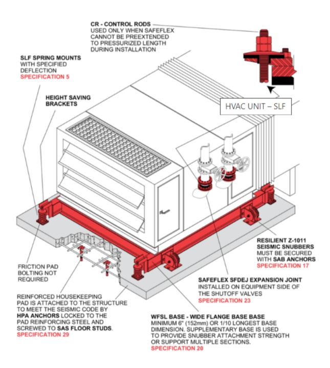
HVAC UNIT directly mounted on 1" deflection SSLFH Spring Mounts. Reinforced housekeeping pad secured by HPA Anchors. SAFEFLEX Expansion Joints are installed in pipelines to reduce blade frequency vibration and noise and to allow for seismic displacement.
