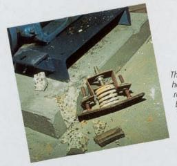
The anchor bolts were too close to the edge of the concrete housekeeping pad for the concrete to offer adequate resistance to the horizontal anchor bolt forces. The edges broke off so the anchor bolts were freed. This total failure of the restraint system occurred at only 0.15qV and 0.15qH. The mountings themselves showed considerable distortion
