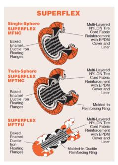
Our engineers never stand still when there is room for improvement and the company moved on to "SUPERFLEX". The SUPERFLEX elastomer was changed from Neoprene to EPDM as most applications are for water service. EPDM is superior to Neoprene in minimizing water swell and resistance to oxygen and ozone aging is outstanding. High temperature tolerance is much better as well.
