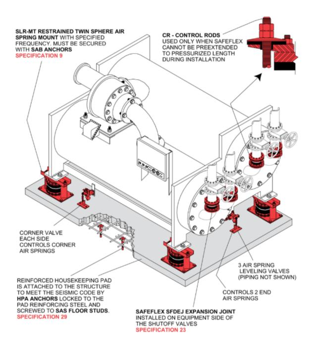
**CENTRIFUGAL CHILLER** on WFSL Base with height saving brackets and high deflection SLF Mounts and Z-1011 Seismic Restraints. Reinforced housekeeping pad secured by HPA Anchors. SAFEFLEX Expansion Joints are installed in pipelines to reduce blade frequency vibration and noise and to allow for seismic displacement.
